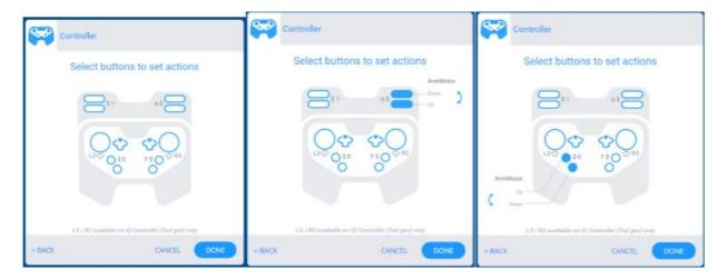
(4) Change the drive mode of the robot by selecting the joysticks
